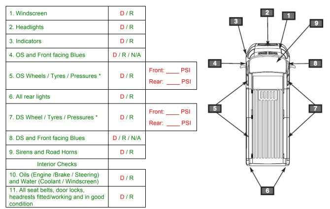
\* Tyres must have 1.6mm tread depth over the centre 3/4 of the tyre and around the entire circumference. There should be no cuts, lumps, bulges, tread separation or sidewall cracking. Tyres must be inflated to the correct pressure (PSI).
